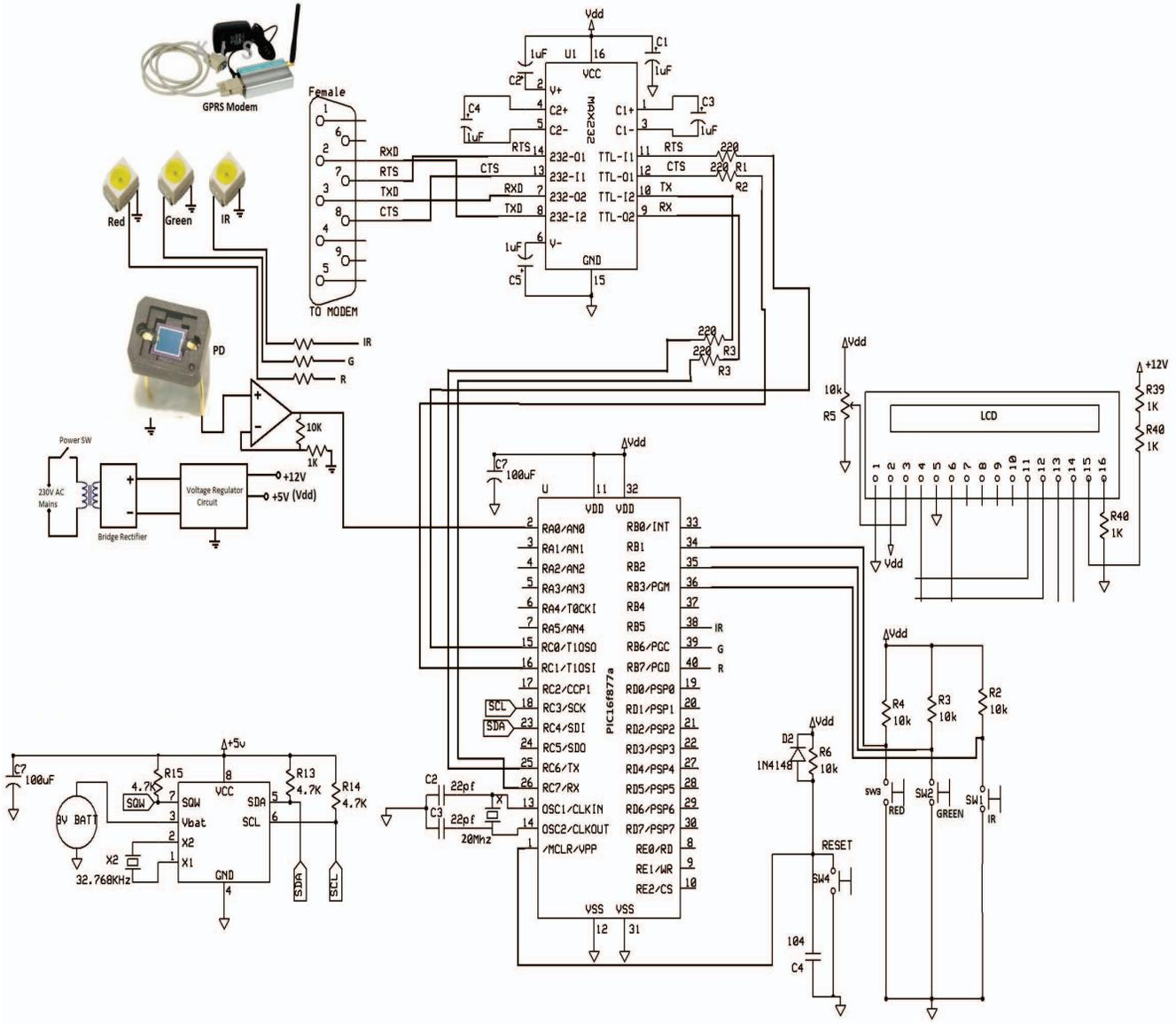
Figure 1. Soil macro-nutrient detection circuit
