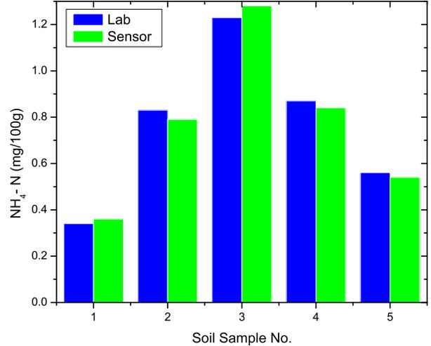
Figure 5. Comparison between lab and sensor data for  $NH_4-N$
