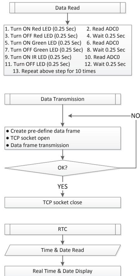
Figure 4. Data reading, data transmission and RTC mechanism
