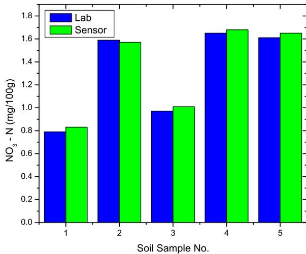
Figure 6. Comparison between lab and sensor data for  $NO_3-N$
