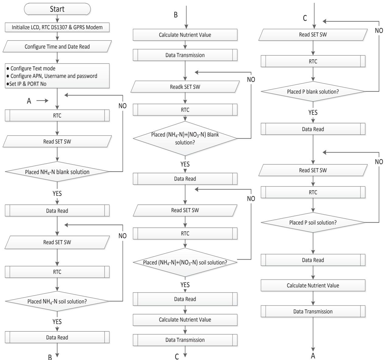
Figure 3. Working procedure of the developed sensing system
