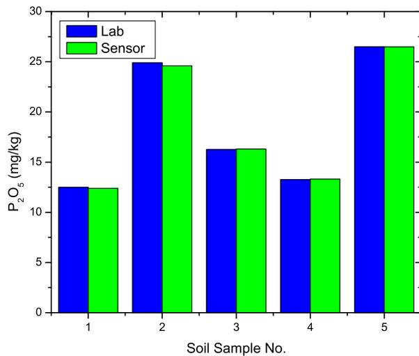
Figure 7. Comparison between lab and sensor data for  $P_2O_5$
