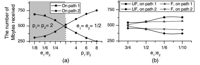
Fig. 2. (a) Trade-off between load-balancing and energy-saving; (b) trade-off between fairness and energy-saving.
