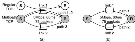
Fig. 3. (a) A three-path ecMTCP flow vs. a regular TCP flow; (b) a two-path ecMTCP/MPTCP flow.
