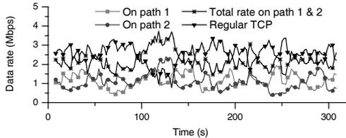
Fig. 4. Fairness with  $e_1 : e_3 = e_2 : e_3 = 1/4$  and a 0.01% packet loss rate on links 1 and 2. The data rate was sampled once every 2 seconds.
