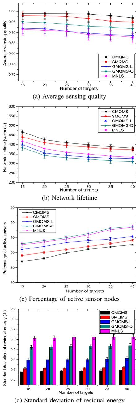
Fig. 7. Impacts of varying targets (area = 500m  $\times$  500m, sensing radius = 50m, number of nodes = 250, sensing sector = 4)
