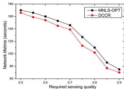
Fig. 1. Impacts of sensing quality on network lifetime (Experiments are conducted in NS-3 [19] with area = 100m × 100m, sensor nodes = 100, sensing radius = 25m, target = 20, sensing sector = 4)
