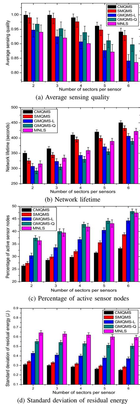
Fig. 9. Impacts of varying sensing sectors (area =  $500\text{m} \times 500\text{m}$ , number of targets = 25, number of nodes = 250, sensing radius = 50m)
