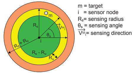
Fig. 2. Probabilistic sensing model
