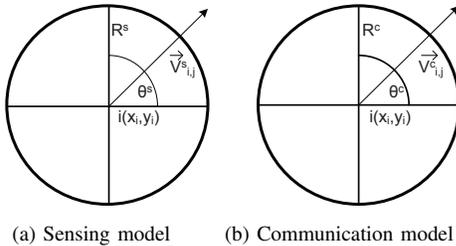
Fig. 1. Sensing and communication models of a directional sensor node
