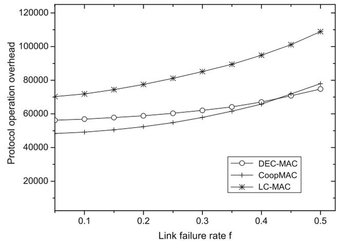
Fig. 15 Protocol operation overhead vs. link failure rate
