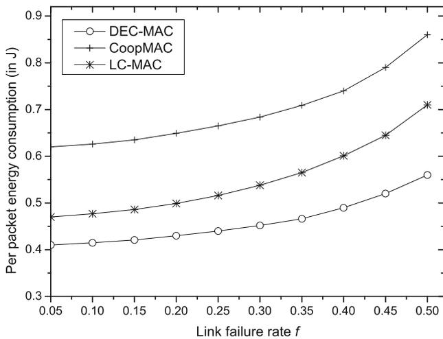
Fig. 13 Energy efficiency vs. link failure rate
