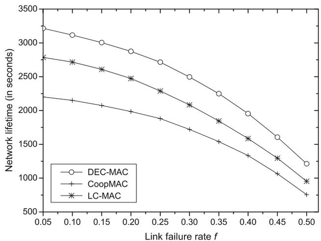
**Fig. 12** Network lifetime vs. link failure rate
