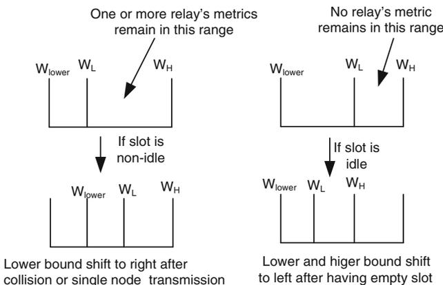
**Fig. 3** Upper and lower threshold update procedure
