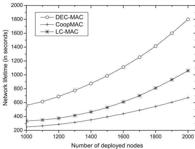
**Fig. 7** Network lifetime vs. number of deployed nodes
