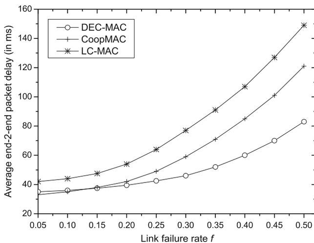
**Fig. 11** Average end-to-end delay vs. link failure rate
