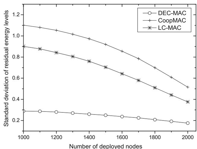
**Fig. 9** Standard deviation of residual energy vs. number of deployed nodes
