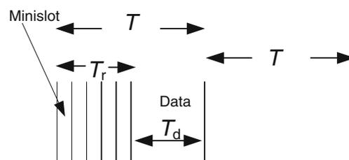
Fig. 2 Time slots for two data bursts
