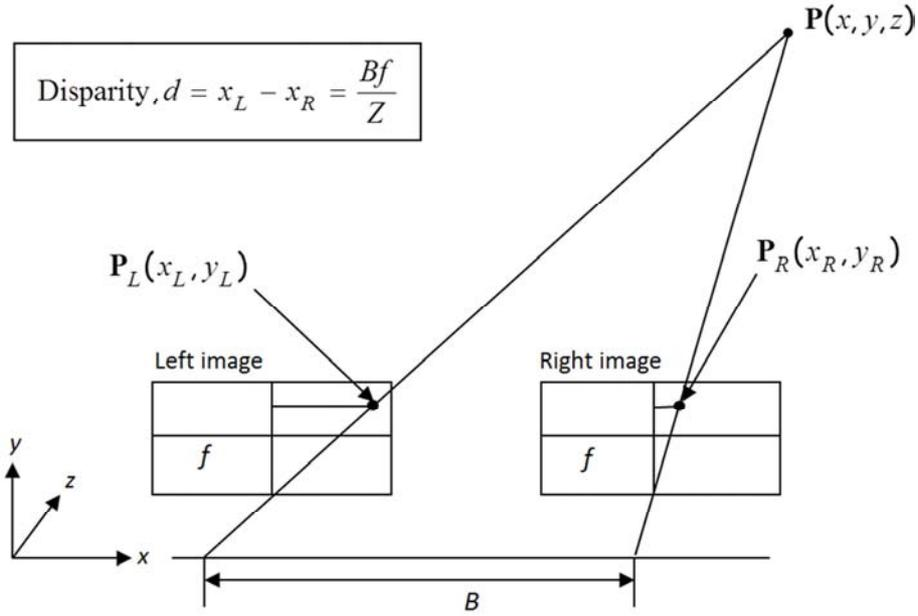
Figure 1. Disparity in a stereo pair of images.
