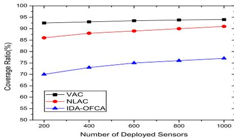
Fig. 5. Coverage percentage vs. number of deployed sensor devices
